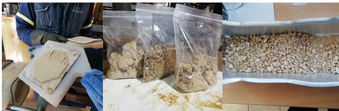
Figure 6. Crude Sc concentrate (22%) produced at MYTILINEOS II-VI pilot plant.
